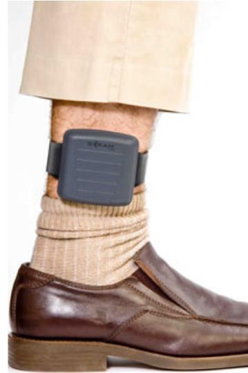
**Fig. 1.** Secure Continuous Remote Alcohol Monitor (SCRAM) bracelet device.
